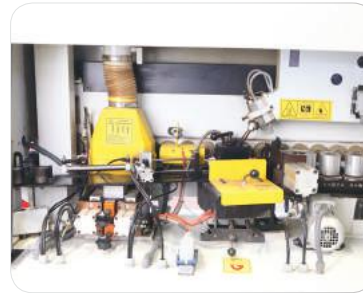
ÖN FREZE, TUTKALLAMA VE BASKI PRE MILLING, GLUE AND PRESS
