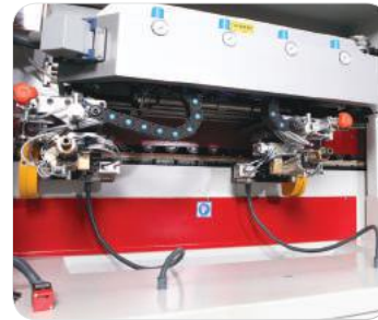
AÇILIR ÖZELLİKLİ BAŞ-SON KESME ANGLE ADJUSTABLE FRONT AND BACK CUTTING UNIT
