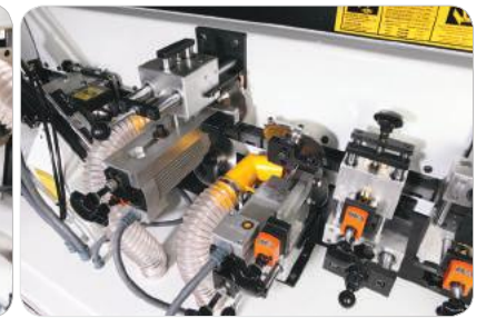
KAZIMA VE POLİSAJ FREZE SCRAPING AND BRUSHING MILLING
