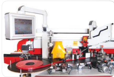
JAMPINGLI ÖN FREZELEME, ÖN ISITICI, SERVO BASKI JUMPING PRE-MILLING UNIT, FRONT HEATER, PRESS
