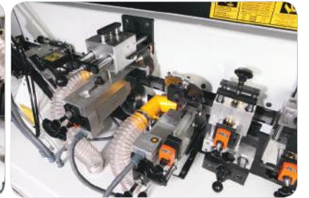
FREZE, KAZIMA VE POLİSAJ MILLING, SCRAPING AND BRUSHING
