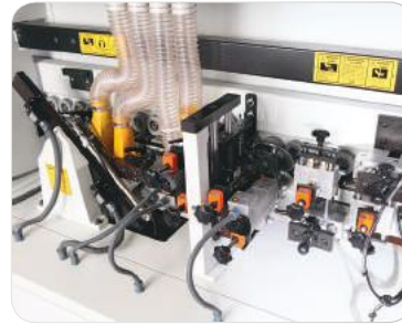
BAŞ SON KESME, FREZE, KAZIMA FIRST END CUTTING, MILLING, SCRAPING
