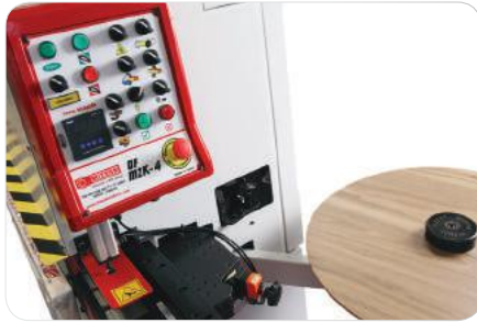
KONTROL PANELİ CONTROL BOARD
